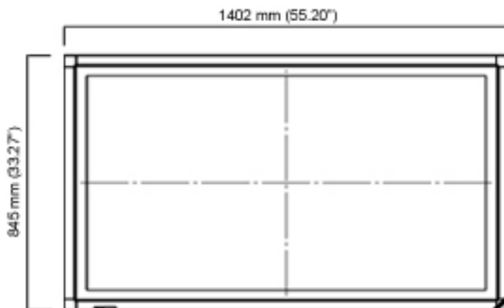
Figure 10: Dimension of BrainSUITE Data Wall Screen 57" - Conrac
